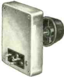
The resistance element is graphite paint, fused to an enameled metal base at high temperature. Pure silver floating contact. Metal cover for rapid heat dissipation.
