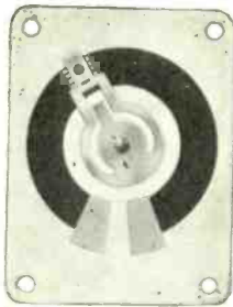
The resistance element is graphite paint, fused to an enameled metal base at high temperature. Pure silver floating contact. Metal cover for rapid heat dissipation.
