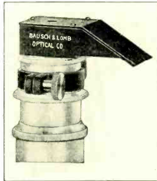
Fig. 25. Illustration of a Camera Lucida.
