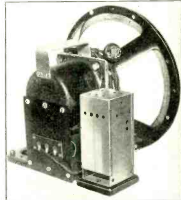
Fig. 1. A dynamic speaker equipped with the high voltage, dry disc rectifier unit.
