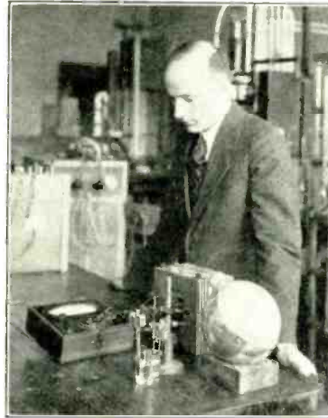
The "Daylight Integrator"—a setup for measuring light over long intervals of time, by means of electrolysis. (Courtesy of General Electric Co.)
